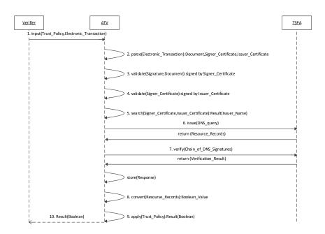
Fig. 2: Sequence Diagram for Trust Publication of a Qualified Signature (Boolean)
