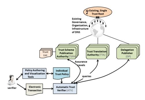
Fig. 1: The LIGHTest Reference Architecture (see also [BL16])
